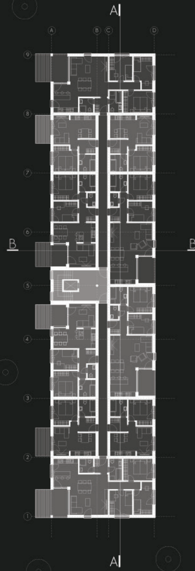
GROUND FLOOR PLAN One bedroom apartment x4 Two bedroom apartment x4 Three bedroom apartment x2
